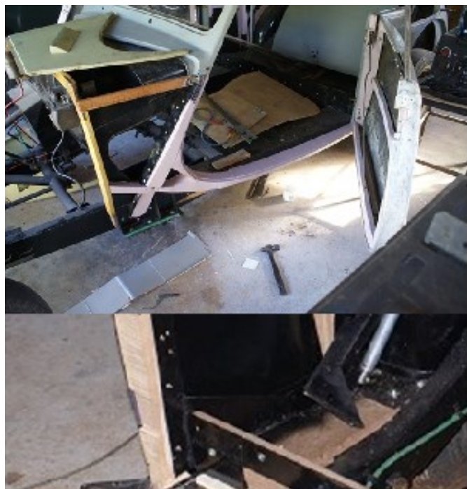
Above: The A pillar is re-enforced with steel
