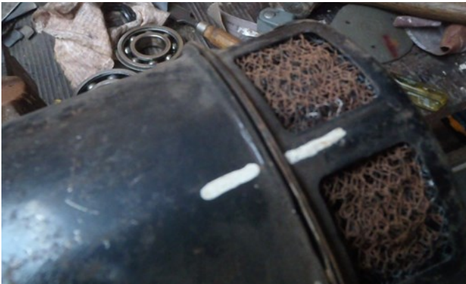
Above: The joint after the grinding operation
