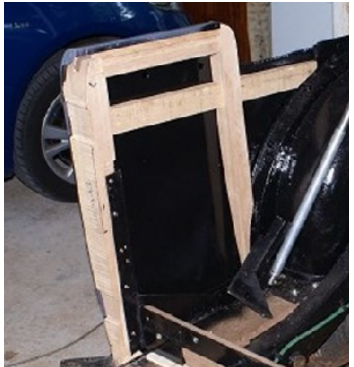
Above: The rear quarter panel in a RMD. You can see the hood assembly piston on the right hand side. The 'B' pillar is re-enforced with a steel that comes down to the rear seat squab and across to the other side of the Riley
