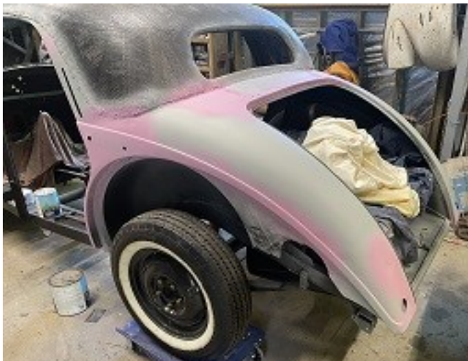
Above: The spots where minor oxidation had eaten the metal surface were filled with pray putty
