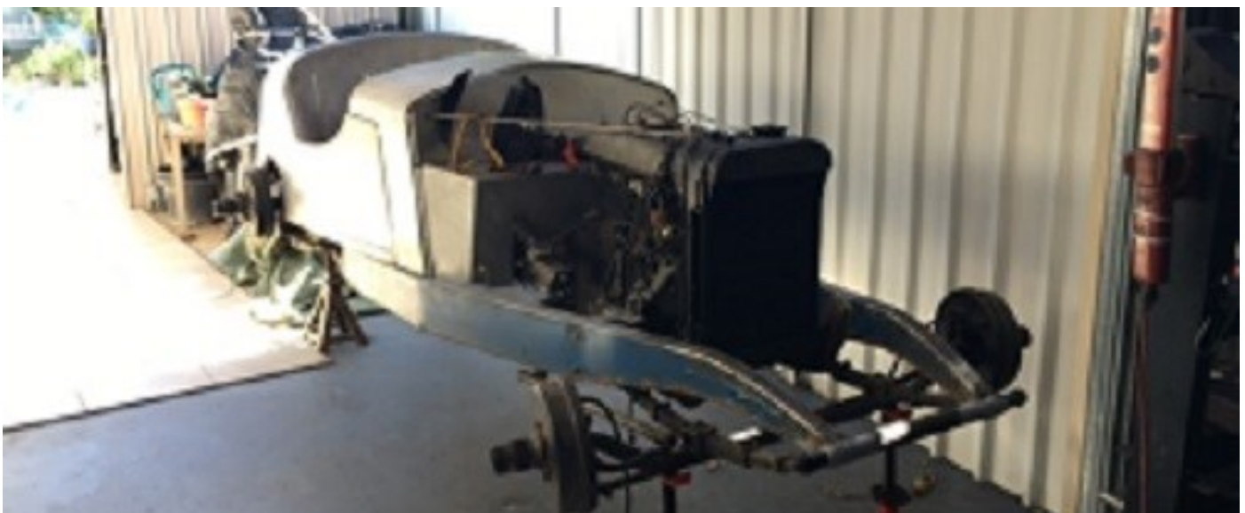
Below: The body refabricated and beginning to look like an Imp.
