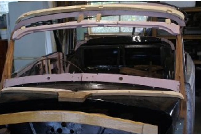
Above: Another view of a top and bottom windscreen rail and the header rail on an RMD.
