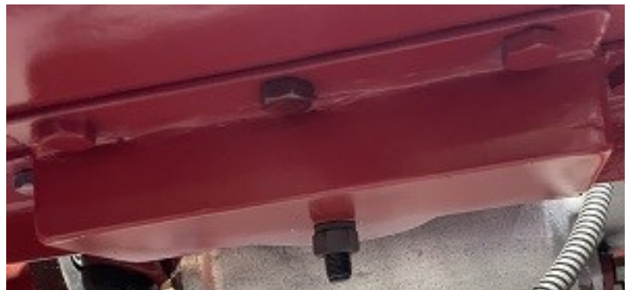
Above: The cradle for the gearbox rubber mounts under the chassis
