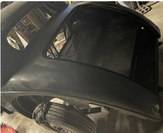
Above: The tub appeared to be straight when the top coat was first applied but when blocked shallow spots and tiny divots were revealed.
