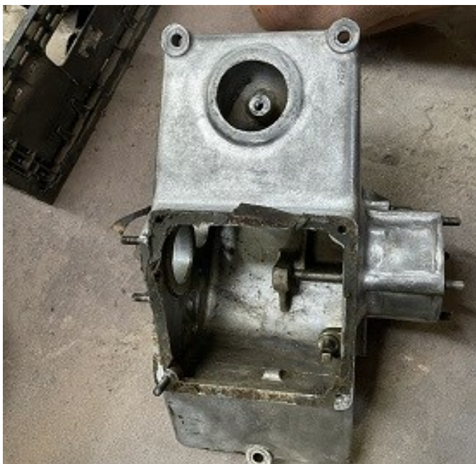
Below: Intact gearbox body. The gears are in the box top left
